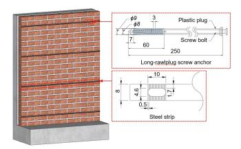
Fig. 1 Schematic of long-rawlplug screw anchor and steel strip
